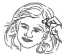
5. Press the START button once and release it. Start to move the instrument steadily from 1cm above the center of the eyebrow to 1cm above the tail of the eyebrow area. A long beep sound will emit after 3 seconds to acknowledge the completion of measurement. If the probe movement is too slow to reach the tail of the eyebrow before the long beep sound heard, repeat the measurement as above from point 4, but simply move the probe a little quicker this time.
